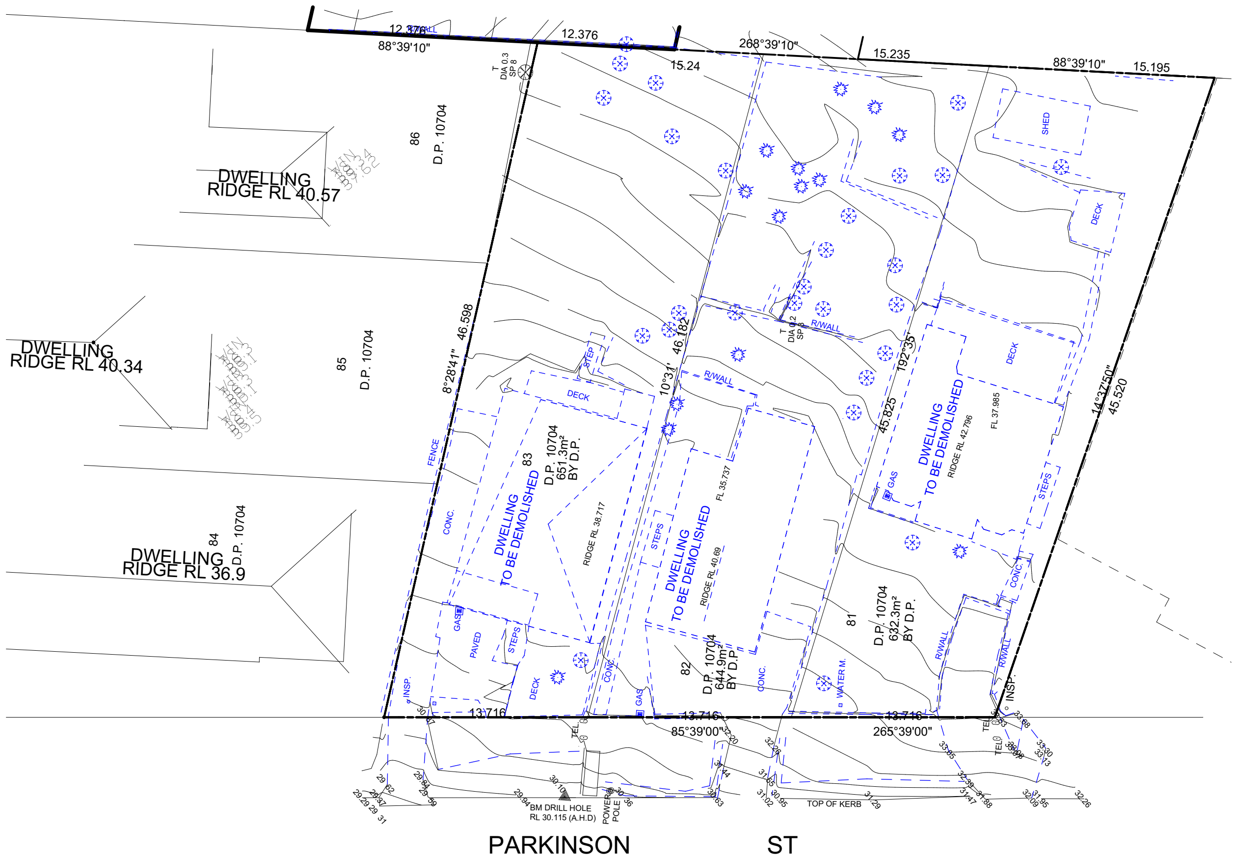
DEMOLITION PLAN SCALE 1:250
